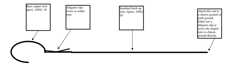
Note: Alligator clips can be the screw type or the solder type.
